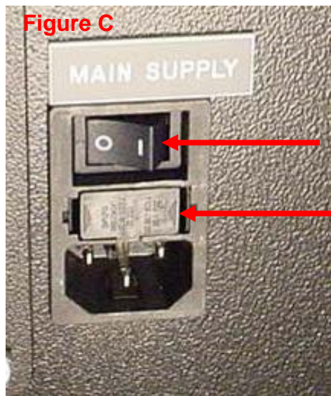
1. Main Supply Power Switch
